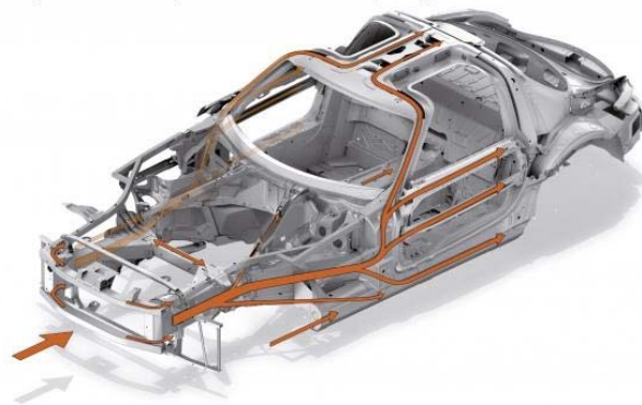
Front impact: the crash load paths are directed around the passengers
