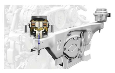
Very soft engine mounts minimise the transmission of vibrations. However, the weight of the engine follows the steering movement with a delay, thus creating unwanted effects when driving very dynamically.
