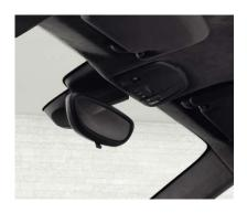
The **light design package** with **dimmable LED ambient lighting** is available as an option. It includes ambient lighting in the overhead console, around the door handles and rear seats, in the door storage boxes and
