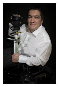
"Hydraulic compression control complements the traditional action of classic, polyurethane bump stops. As its absorption capabilities are significantly improved, it can react later to wheel movements. The suspension thus performs in a much more linear manner that has two main benefits: - obstacles and poor road surfaces are much better absorbed, without any 'rebound' effect.
