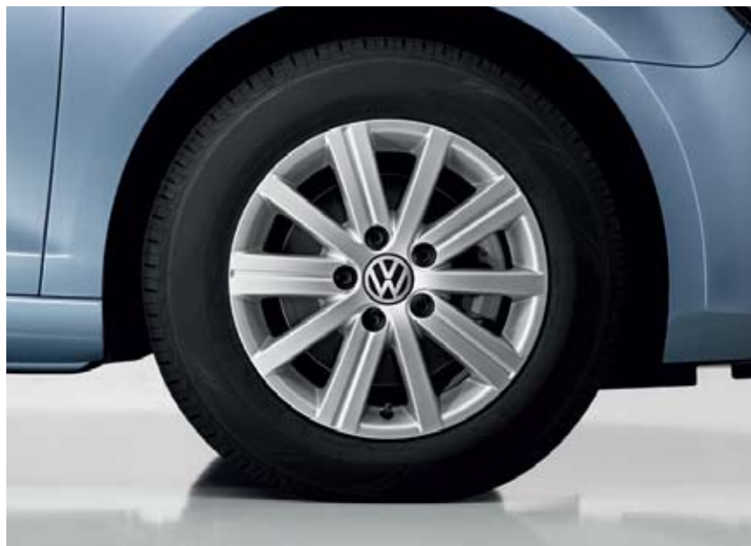
'Wellington' 6J x 15 light alloy wheels with 195/65 R15 tyres. Optional on S models.
