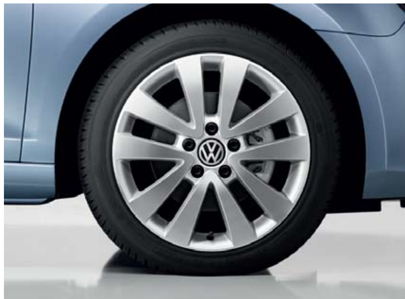
'Seattle' 7J x 17 light alloy wheels with 225/45 R17 tyres. Optional on GT models.
